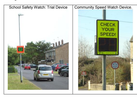
SSW devices cost approximately £2000 each. This is similar to the CSW signs. Both signs are powered by rechargeable batteries.
